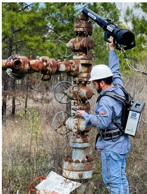
Figure 39. A DOE employee measures methane from an orphaned well in Texas. Photo taken by the USFS.
