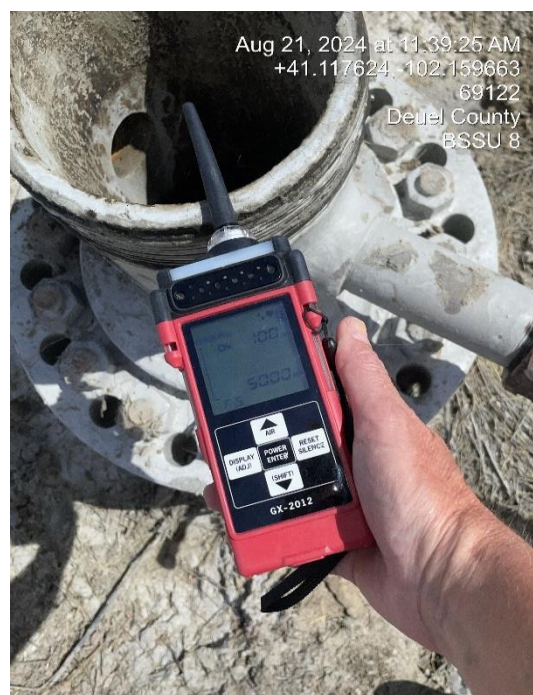
Figure 40. Using equipment to conduct a methane detection test at a well in Nebraska.
